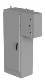
Saginaw enclosure, NEMA 3R/12/13, 72 x 34 x 18in (HxWxD), freestanding, carbon steel, ANSI 61 gray, powder coat finish, single-door, 3-point padlocking handle, external rotary disconnect enclosure included.
