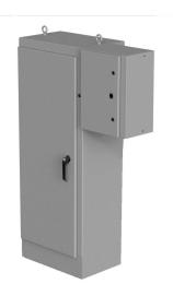
Saginaw enclosure, NEMA 3R/12/13, 72 x 34 x 18in (HxWxD), freestanding, carbon steel, ANSI 61 gray, powder coat finish, single-door, 3-point padlocking handle, external rotary disconnect enclosure included.
