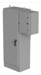
Saginaw enclosure, NEMA 3R/12/13, 72 x 34 x 18in (HxWxD), freestanding, carbon steel, ANSI 61 gray, powder coat finish, single-door, 3-point padlocking handle, subpanel and external rotary disconnect enclosure included.
