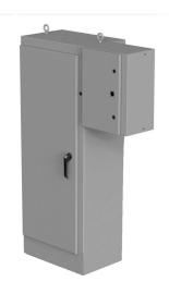
Saginaw enclosure, NEMA 3R/4/12/13, 72 x 28 x 18in (HxWxD), freestanding, carbon steel, ANSI 61 gray, powder coat finish, single-door, 3-point padlocking handle, external rotary disconnect enclosure included.
