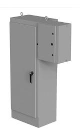
Saginaw enclosure, NEMA 3R/4/12/13, 72 x 28 x 18in (HxWxD), freestanding, carbon steel, ANSI 61 gray, powder coat finish, single-door, 3-point padlocking handle, subpanel and external rotary disconnect enclosure included.
