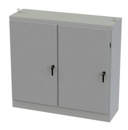
Saginaw disconnect enclosure, NEMA 3R/12/13, right flange,  $72 \times 78 \times 24$ in (HxWxD), freestanding, carbon steel, ANSI 61 gray, powder coat finish, 2-door, 3-point padlocking handle, powder coated subpanel included.
