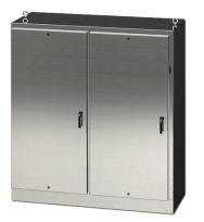
Saginaw disconnect enclosure, NEMA 3R/4/4X/12/13, right flange, 72 x 78 x 24in (HxWxD), freestanding, 304 stainless steel, #4 brush finish, 2-door, 3-point padlocking handle, powder coated subpanel included.
