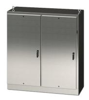
Saginaw disconnect enclosure, NEMA 3R/4/4X/12/13, right flange, 72 x 78 x 18in (HxWxD), freestanding, 316L stainless steel, #4 brush finish, 2-door, 3-point padlocking handle, powder coated subpanel included.
