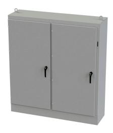
Saginaw disconnect enclosure, NEMA 3R/12/13, right flange,  $72 \times 66 \times 18$  in (HxWxD), freestanding, carbon steel, ANSI 61 gray, powder coat finish, 2-door, 3-point padlocking handle, powder coated subpanel included.
