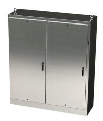
Saginaw disconnect enclosure, NEMA 3R/4/4X/12/13, right flange, 72 x 66 x 18in (HxWxD), freestanding, 316L stainless steel, #4 brush finish, 2-door, 3-point padlocking handle, powder coated subpanel included.
