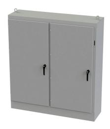
Saginaw disconnect enclosure, NEMA 3R/12/13, right flange, 72 x 66 x 18in (HxWxD), freestanding, carbon steel, ANSI 61 gray, powder coat finish, 2-door, 3-point padlocking handle, galvanized subpanel included.
