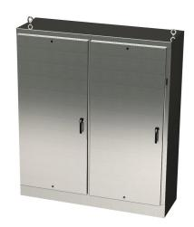
Saginaw disconnect enclosure, NEMA 3R/4/4X/12/13, right flange, 72 x 54 x 18in (HxWxD), freestanding, 304 stainless steel, #4 brush finish, 2-door, 3-point padlocking handle, powder coated subpanel included.
