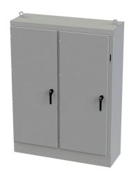
Saginaw disconnect enclosure, NEMA 3R/4/12/13, right flange, 72 x 54 x 18in (HxWxD), freestanding, carbon steel, ANSI 61 gray, powder coat finish, 2-door, 3-point padlocking handle, galvanized subpanel included.
