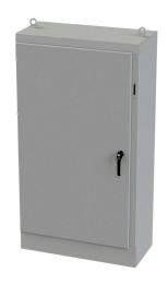
Saginaw disconnect enclosure, NEMA 3R/12/13, right flange,  $72 \times 40 \times 18$  in (HxWxD), freestanding, carbon steel, ANSI 61 gray, powder coat finish, single-door, 3-point padlocking handle, powder coated subpanel included.
