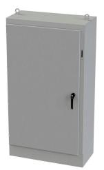
Saginaw disconnect enclosure, NEMA 3R/12/13, right flange, 72 x 40 x 18in (HxWxD), freestanding, carbon steel, ANSI 61 gray, powder coat finish, single-door, 3-point padlocking handle, galvanized subpanel included.
