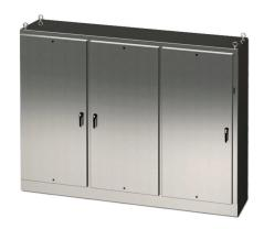
Saginaw disconnect enclosure, NEMA 3R/4/4X/12/13, right flange, 72 x 118 x 18in (HxWxD), freestanding, 304 stainless steel, #4 brush finish, 3-door, 3-point padlocking handle, (2) powder coated subpanels included.
