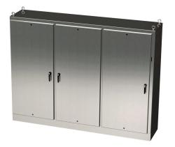
Saginaw disconnect enclosure, NEMA 3R/4/4X/12/13, right flange, 72 x 118 x 18in (HxWxD), freestanding, 316L stainless steel, #4 brush finish, 3-door, 3-point padlocking handle, (2) powder coated subpanels included.
