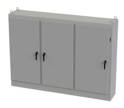
Saginaw disconnect enclosure, NEMA 3R/12/13, right flange,  $72 \times 100 \times 18$  in (HxWxD), freestanding, carbon steel, ANSI 61 gray, powder coat finish, 3-door, 3-point padlocking handle, (2) powder coated subpanels included.
