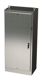
Saginaw disconnect enclosure, NEMA 3R/4/4X/12/13, right flange, 72 x 34 x 18in (HxWxD), freestanding, 316L stainless steel, #4 brush finish, single-door, 3-point padlocking handle, powder coated subpanel included.
