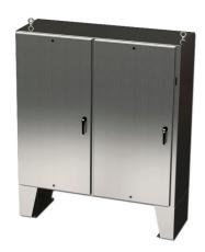
Saginaw Enviroline series disconnect enclosure, NEMA 3R/4/4X/12/13, right flange, 72 x 73 x 24in (HxWxD), floor mount, 304 stainless steel, #4 brush finish, 2-door, 3-point padlocking handle, purchase subpanel separately.
