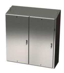
Saginaw Enviroline series disconnect enclosure, slope top, NEMA 3R/4/4X/12/13, right flange, 72 x 73 x 24in (HxWxD), freestanding, 316L stainless steel, #4 brush finish, 2-door, 3-point 304 stainless steel padlocking handle, purchase subpanel separately.
