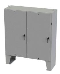
Saginaw Enviroline series disconnect enclosure, NEMA 3R/4/12/13, right flange, 72 x 73 x 24in (HxWxD), floor mount, carbon steel, ANSI 61 gray, powder coat finish, 2-door, 3-point padlocking handle, purchase subpanel separately.
