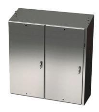
Saginaw Enviroline series disconnect enclosure, slope top, NEMA 3R/4/4X/12/13, right flange, 72 x 73 x 18in (HxWxD), freestanding, 304 stainless steel, #4 brush finish, 2-door, 3-point 304 stainless steel padlocking handle, purchase subpanel separately.
