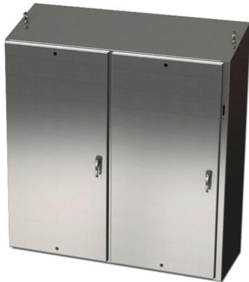
Saginaw Enviroline series disconnect enclosure, slope top, NEMA 3R/4/4X/12/13, right flange, 72 x 73 x 18in (HxWxD), freestanding, 316L stainless steel, #4 brush finish, 2-door, 3-point 304 stainless steel padlocking handle, purchase subpanel separately.
