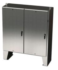
Saginaw Enviroline series disconnect enclosure, NEMA 3R/4/4X/12/13, right flange, 72 x 73 x 12in (HxWxD), floor mount, 304 stainless steel, #4 brush finish, 2-door, 3-point padlocking handle, purchase subpanel separately.
