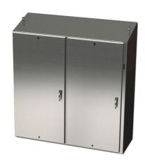
Saginaw Enviroline series disconnect enclosure, slope top, NEMA 3R/4/4X/12/13, right flange, 72 x 73 x 12in (HxWxD), freestanding, 316L stainless steel, #4 brush finish, 2-door, 3-point 304 stainless steel padlocking handle, purchase subpanel separately.
