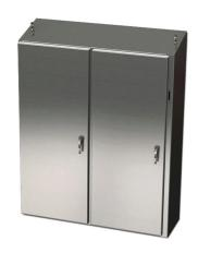
Saginaw Enviroline series disconnect enclosure, slope top, NEMA 3R/4/4X/12/13, right flange, 72 x 61 x 18in (HxWxD), freestanding, 316L stainless steel, #4 brush finish, 2-door, 3-point 304 stainless steel padlocking handle, purchase subpanel separately.
