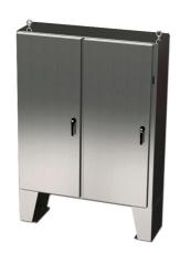
Saginaw Enviroline series disconnect enclosure, NEMA 3R/4/4X/12/13, right flange, 72 x 61 x 18in (HxWxD), floor mount, 316L stainless steel, #4 brush finish, 2-door, 3-point padlocking handle, purchase subpanel separately.
