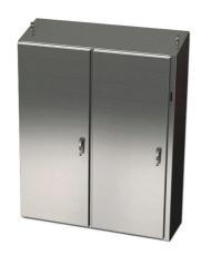
Saginaw Enviroline series disconnect enclosure, slope top, NEMA 3R/4/4X/12/13, right flange, 72 x 61 x 12in (HxWxD), freestanding, 304 stainless steel, #4 brush finish, 2-door, 3-point 304 stainless steel padlocking handle, purchase subpanel separately.
