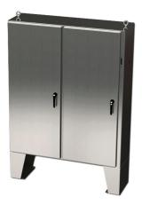
Saginaw Enviroline series disconnect enclosure, NEMA 3R/4/4X/12/13, right flange, 72 x 61 x 12in (HxWxD), floor mount, 304 stainless steel, #4 brush finish, 2-door, 3-point padlocking handle, purchase subpanel separately.
