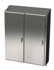
Saginaw Enviroline series disconnect enclosure, slope top, NEMA 3R/4/4X/12/13, right flange, 72 x 61 x 12in (HxWxD), freestanding, 316L stainless steel, #4 brush finish, 2-door, 3-point 304 stainless steel padlocking handle, purchase subpanel separately.
