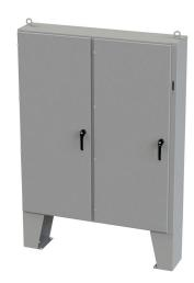
Saginaw Enviroline series disconnect enclosure, NEMA 3R/4/12/13, right flange, 72 x 61 x 12in (HxWxD), floor mount, carbon steel, ANSI 61 gray, powder coat finish, 2-door, 3-point padlocking handle, purchase subpanel separately.
