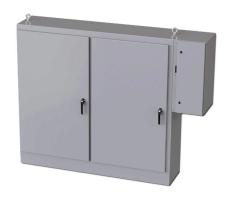
Saginaw enclosure, NEMA 3R/12/13, 72 x 78 x 18in (HxWxD), freestanding, carbon steel, ANSI 61 gray, powder coat finish, 2-door, 3-point padlocking handle, external disconnect enclosure included.
