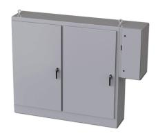
Saginaw enclosure, NEMA 3R/12/13, 72 x 78 x 18in (HxWxD), freestanding, carbon steel, ANSI 61 gray, powder coat finish, 2-door, 3-point padlocking handle, subpanel and external disconnect enclosure included.
