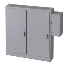
Saginaw enclosure, NEMA 3R/12/13, 72 x 66 x 18in (HxWxD), freestanding, carbon steel, ANSI 61 gray, powder coat finish, 2-door, 3-point padlocking handle, external disconnect enclosure included.
