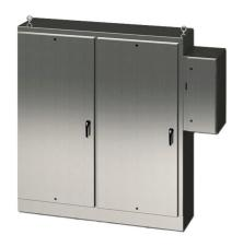
Saginaw enclosure, NEMA 3R/4/4X/12/13, 72 x 66 x 18in (HxWxD), freestanding, 316L stainless steel, #4 brush finish, 2-door, 3-point padlocking handle, external disconnect enclosure included.
