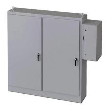
Saginaw enclosure, NEMA 3R/12/13, 72 x 66 x 18in (HxWxD), freestanding, carbon steel, ANSI 61 gray, powder coat finish, 2-door, 3-point padlocking handle, subpanel and external disconnect enclosure included.
