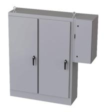
Saginaw enclosure, NEMA 3R/4/12/13, 72 x 54 x 18in (HxWxD), freestanding, carbon steel, ANSI 61 gray, powder coat finish, 2-door, 3-point padlocking handle, subpanel and external disconnect enclosure included.
