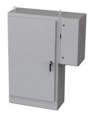
Saginaw enclosure, NEMA 3R/12/13, 72 x 40 x 18in (HxWxD), freestanding, carbon steel, ANSI 61 gray, powder coat finish, single-door, 3-point padlocking handle, external disconnect enclosure included.
