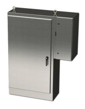
Saginaw enclosure, NEMA 3R/4/4X/12/13, 72 x 40 x 18in (HxWxD), freestanding, 316L stainless steel, #4 brush finish, single-door, 3-point padlocking handle, external disconnect enclosure included.
