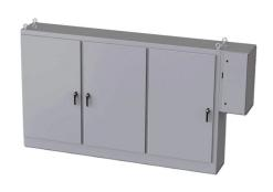
Saginaw enclosure, NEMA 3R/12/13, 72 x 118 x 18in (HxWxD), freestanding, carbon steel, ANSI 61 gray, powder coat finish, 3-door, 3-point padlocking handle, external disconnect enclosure included.
