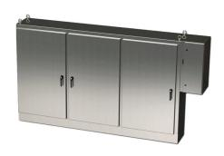
Saginaw enclosure, NEMA 3R/4/4X/12/13, 72 x 118 x 18in (HxWxD), freestanding, 304 stainless steel, #4 brush finish, 3-door, 3-point padlocking handle, external disconnect enclosure included.
