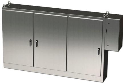
Saginaw enclosure, NEMA 3R/4/4X/12/13, 72 x 118 x 18in (HxWxD), freestanding, 304 stainless steel, #4 brush finish, 3-door, 3-point padlocking handle, external disconnect enclosure included.
