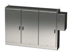
Saginaw enclosure, NEMA 3R/4/4X/12/13, 72 x 118 x 18in (HxWxD), freestanding, 316L stainless steel, #4 brush finish, 3-door, 3-point padlocking handle, external disconnect enclosure included.
