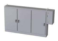
Saginaw enclosure, NEMA 3R/12/13, 72 x 118 x 18in (HxWxD), freestanding, carbon steel, ANSI 61 gray, powder coat finish, 3-door, 3-point padlocking handle, subpanel and external disconnect enclosure included.
