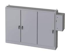
Saginaw enclosure, NEMA 3R/12/13, 72 x 100 x 18in (HxWxD), freestanding, carbon steel, ANSI 61 gray, powder coat finish, 3-door, 3-point padlocking handle, external disconnect enclosure included.
