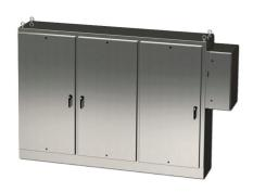
Saginaw enclosure, NEMA 3R/4/4X/12/13, 72 x 100 x 18in (HxWxD), freestanding, 316L stainless steel, #4 brush finish, 3-door, 3-point padlocking handle, external disconnect enclosure included.
