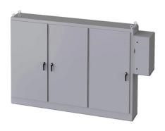
Saginaw enclosure, NEMA 3R/12/13, 72 x 100 x 18in (HxWxD), freestanding, carbon steel, ANSI 61 gray, powder coat finish, 3-door, 3-point padlocking handle, subpanel and external disconnect enclosure included.
