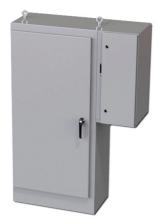
Saginaw enclosure, NEMA 3R/12/13, 72 x 34 x 18in (HxWxD), freestanding, carbon steel, ANSI 61 gray, powder coat finish, single-door, 3-point padlocking handle, external disconnect enclosure included.
