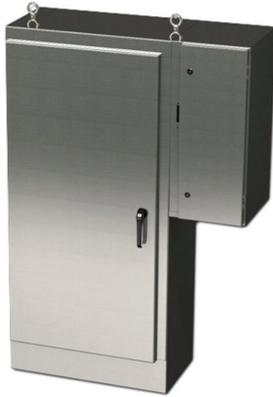
Saginaw enclosure, NEMA 3R/4/4X/12/13, 72 x 34 x 18in (HxWxD), freestanding, 304 stainless steel, #4 brush finish, single-door, 3-point padlocking handle, external disconnect enclosure included.
