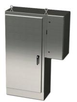
Saginaw enclosure, NEMA 3R/4/4X/12/13, 72 x 34 x 18in (HxWxD), freestanding, 304 stainless steel, #4 brush finish, single-door, 3-point padlocking handle, external disconnect enclosure included.
