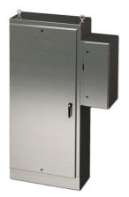
Saginaw enclosure, NEMA 3R/4/4X/12/13, 72 x 34 x 18in (HxWxD), freestanding, 316L stainless steel, #4 brush finish, single-door, 3-point padlocking handle, external disconnect enclosure included.
