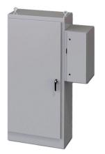
Saginaw enclosure, NEMA 3R/12/13, 72 x 34 x 18in (HxWxD), freestanding, carbon steel, ANSI 61 gray, powder coat finish, single-door, 3-point padlocking handle, subpanel and external disconnect enclosure included.
